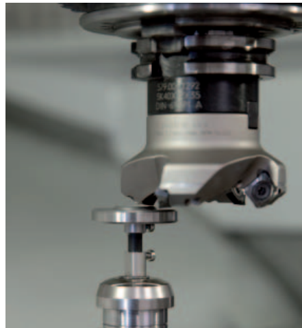
Tool wear measurement and tool breakage monitoring
