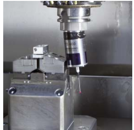
TS 460 with collision protection
